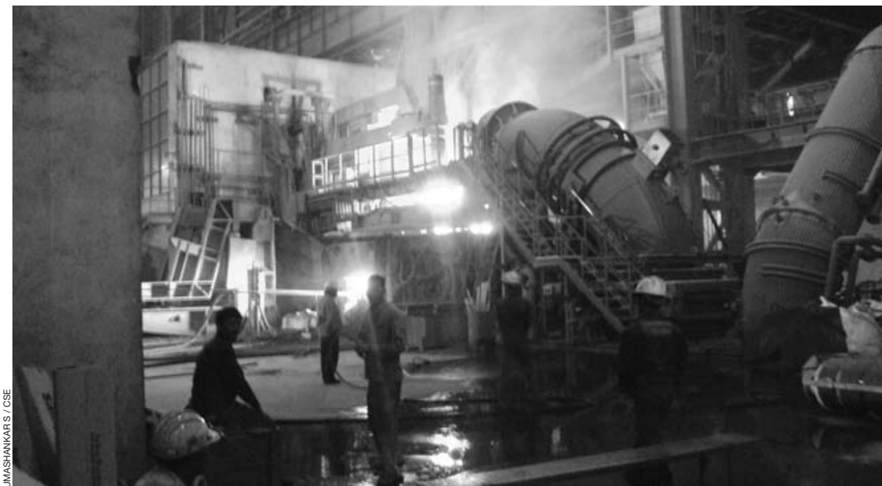
Secondary emissions release from arc furnace operation at Bhushan Power and Steel, Sambalpur
